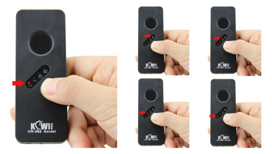
4. Then press the shutter button on UR-262 to enable the function you choose in step 3. When you press the shutter button of the UR-262, the specific function led light will flash.
