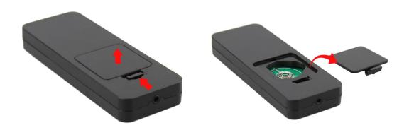
2. Insert a CR-2032 battery to the battery compartment with anode facing upwards and press down. Make sure battery is well installed into the battery compartment for use. Do not install batteries in the reverse direction as this could cause the batteries to leak corrosive liquids, generate heat or explode.
